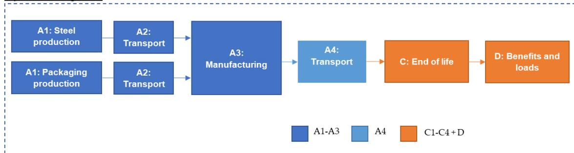
Steel and packaging materials are transported to a manufacturing plant where the stainless acid proof wall ties are manufactured. In this plant the steel is bent, cut and punched (all dry operations) to different shapes and sizes depending on which product that are manufactured. The wall ties are then distributed to the final customers. After use the product is transported to waste processing, and the steel is recycled.
